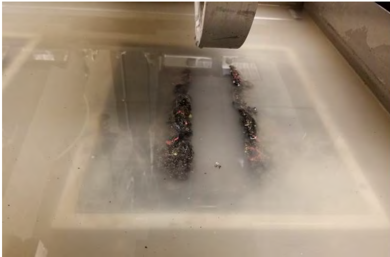
Figure 6—Example of Muddy Water after Performing Hamburg Test
