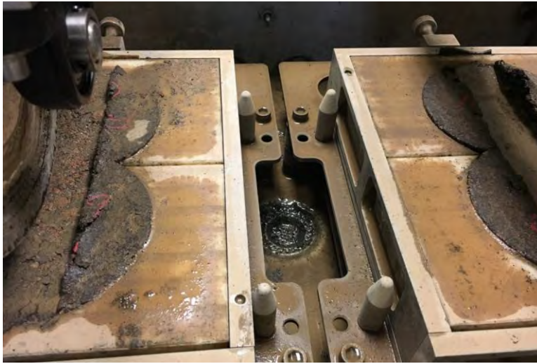
Figure 5—Example of Excessive Fines in the Water Bath
